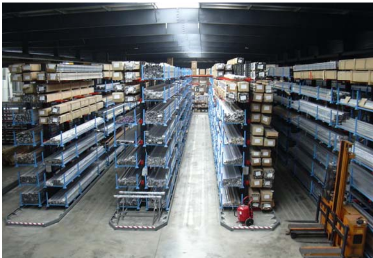
Fig. 1: Round material in cassettes to assist in transport and storage—ELVEDI cantilever racking over 9 m high for loads up to 20 tons per column and side.
