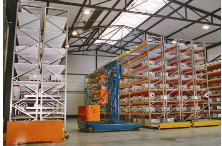
ELVEDI double depth pallet racking equipped with grid for storage of pallets and small parts.
