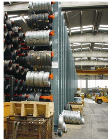
Fig. 2: Wire coils held by a cantilever arm with a length of 2000 mm and load capacity of 1000 kg per arm.
