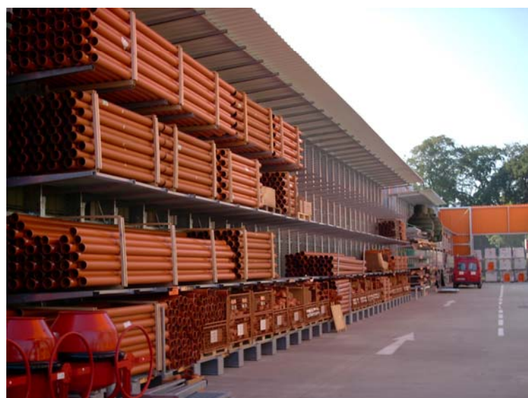
Open-air storage for weatherproof products - Cantilever equipped with roll off protection
